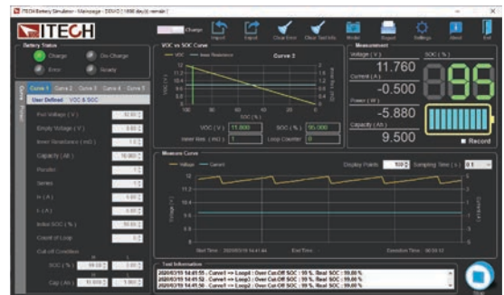
BSS2000 battery emulation software interface
