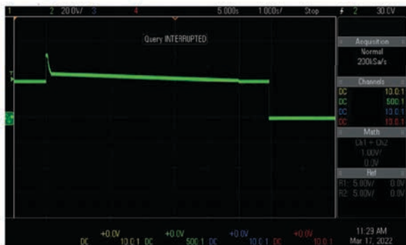
LDC302 28V abnormal voltage transients (overvoltage)
